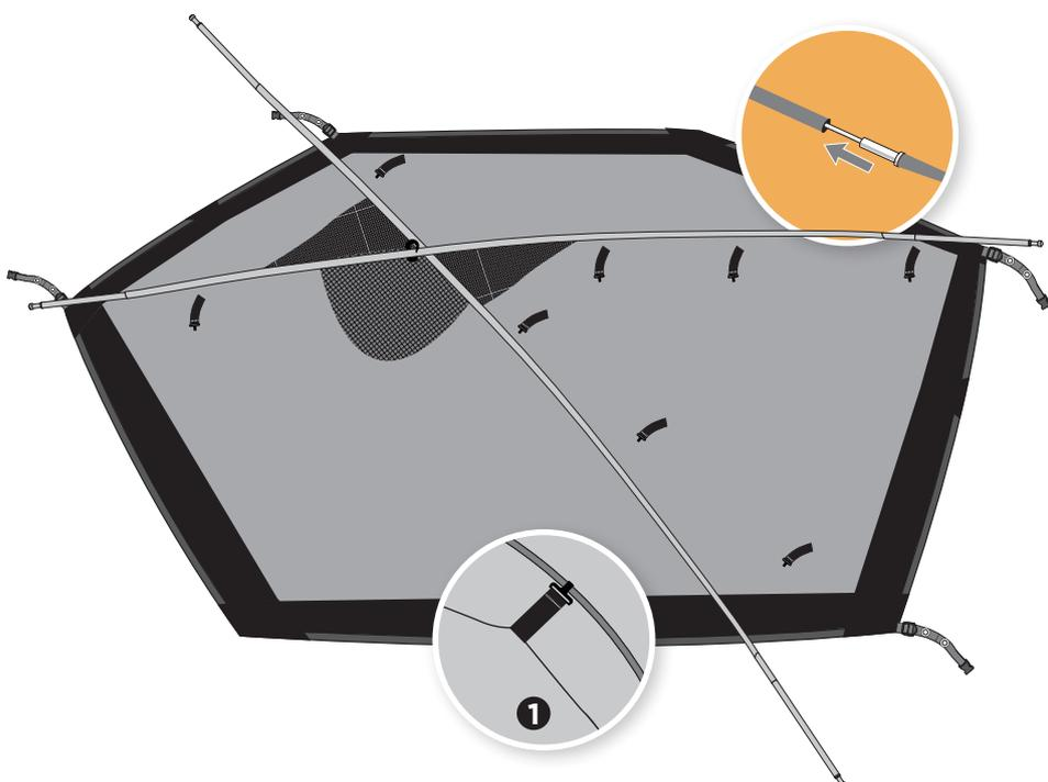
Lay out the footprint before erecting the tent. Unroll the inner tent and locate the pole bag, separate the poles, clip the sections together making continuous poles. The poles are held together by elastic.
