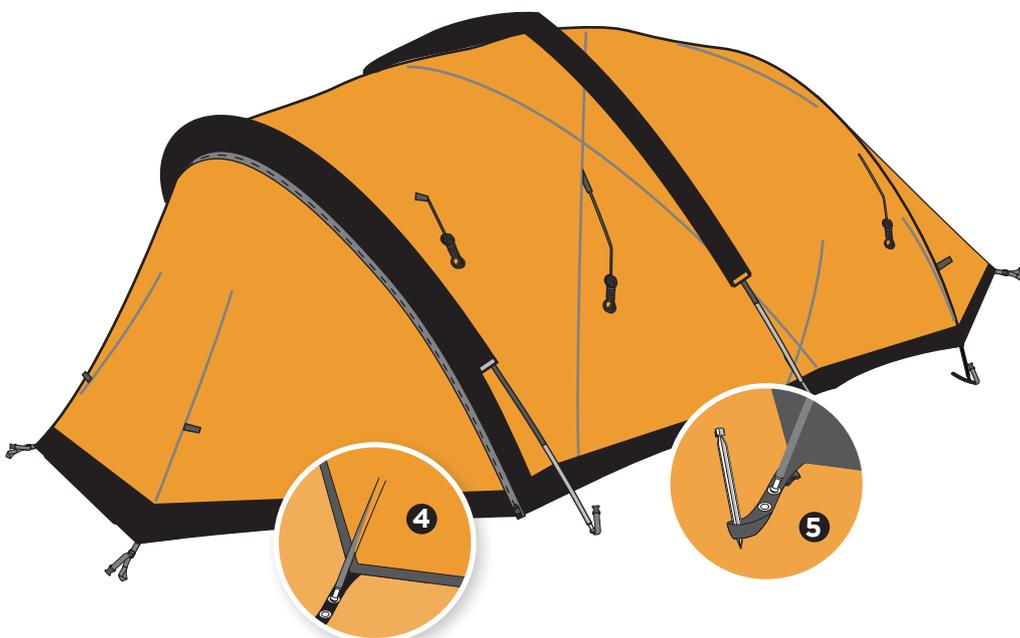
4. Insert the pole ends into the grommets in the corresponding webbing straps.
