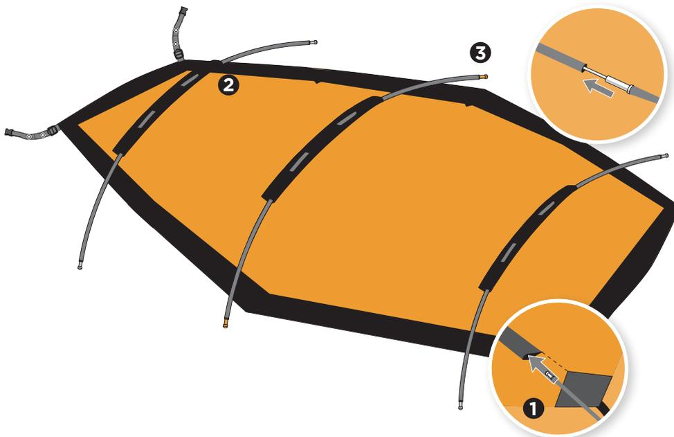
Lay out the footprint before erecting the tent. Unroll the outer tent, locate the pole bag, separate the poles, clip the sections together making continuous poles. The poles are held together by elastic.
